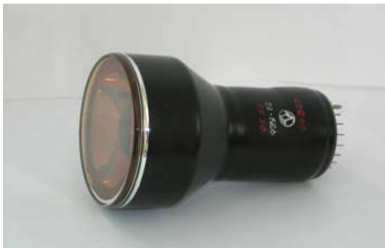
Fig. 6 General view of the 12-dynode spectroscopic photomultiplier tube PMT-82.
