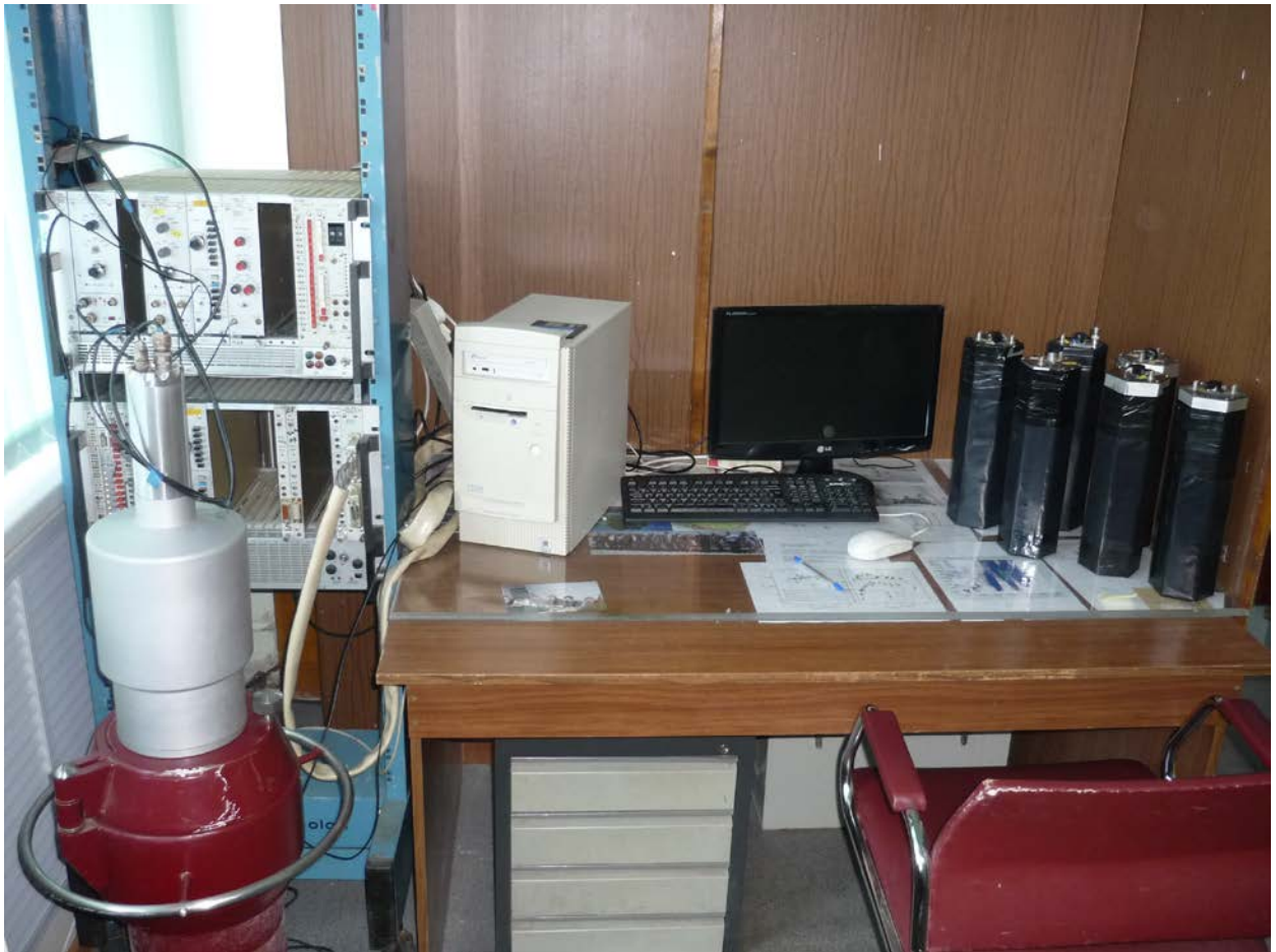
Fig. 7 General view of a single-crystal \gamma -radiation scintillation spectrometer.
