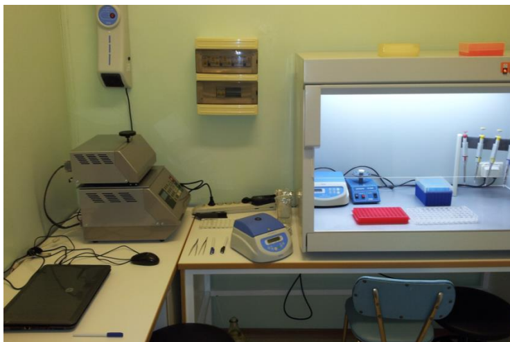
Fig. 4 – Laboratory room, with PCR box and PCR amplifier, where the DNA samples are isolated, measured and prepared for further analysis.
