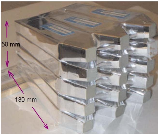
Fig. 2. Electromagnetic calorimeter prototype.
