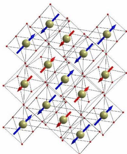
**Figure 1.** The schematic representation of a magnetic structure of  $\text{Pb}_2\text{FeSbO}_6$  compound at low temperatures. The iron atoms inside oxygen octahedra and corresponding magnetic moments are shown. The blue and red arrows mark the magnetic moments of Fe ions in crystallographic iron site  $(0, 0, 0)$  and antimony site  $(0, 0, \frac{1}{2})$  respectively.
