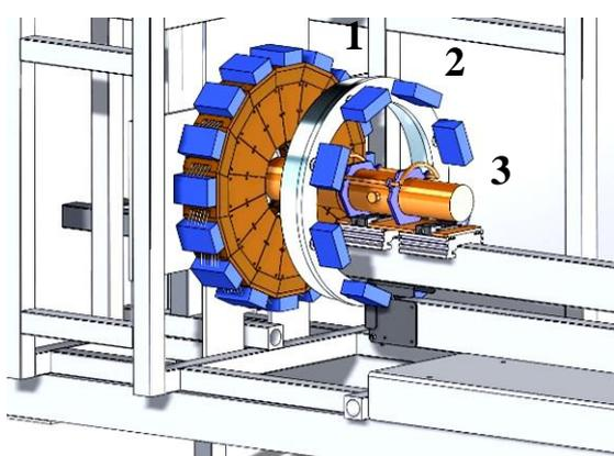
*Figure 2. Enlarged schematic layout of detector and sample environment systems of the DN-6 diffractometer. The 90-deg. scattering angle detector section (1), the low scattering angle detector section (2), the horizontal cryostat (3) and sample and high-pressure cells holders fixed on the movable slider are shown. The diffractometer components are mounted on a mechanical support cage.*
