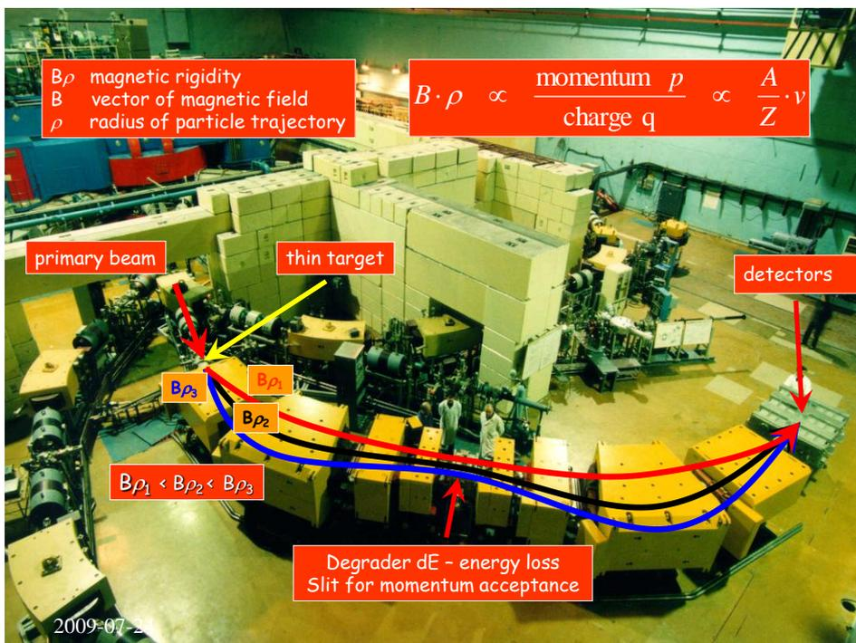
Fig.1 General view of the COMBAS fragment separator installed in the experimental hall of the U-400M cyclotron of the FLNR at the JINR.
